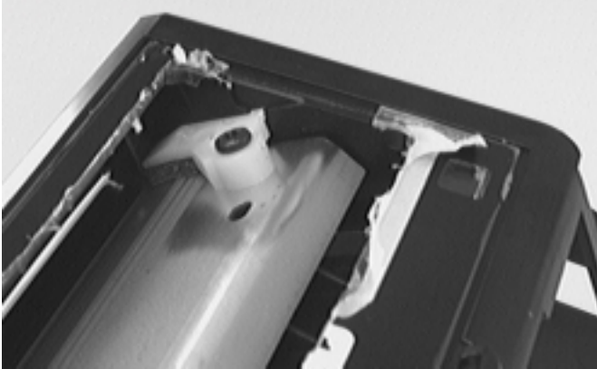
Fig. 3. Cut-out in toner-cartridge cover to access mounting screws.
