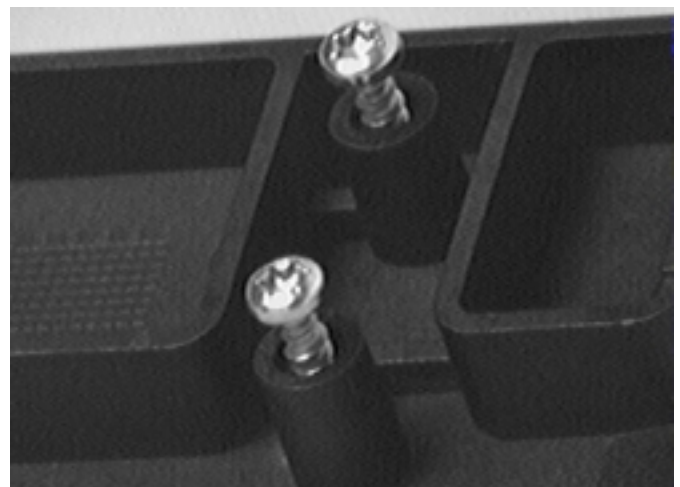
Fig. 2. Thread-forming screws used to fasten paper guide to base.
