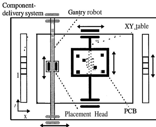
Figure 1: The generalized electronic-component-placement machine configuration.
