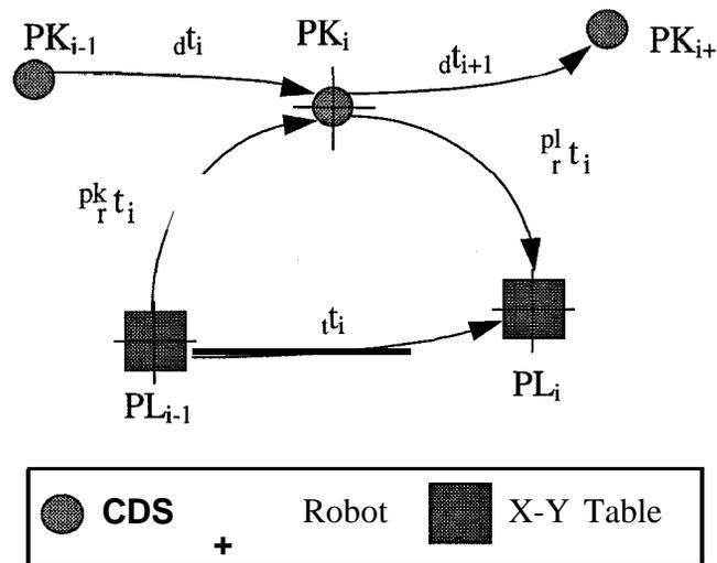
Figure 2: Illustration of cyclic device motion times.
