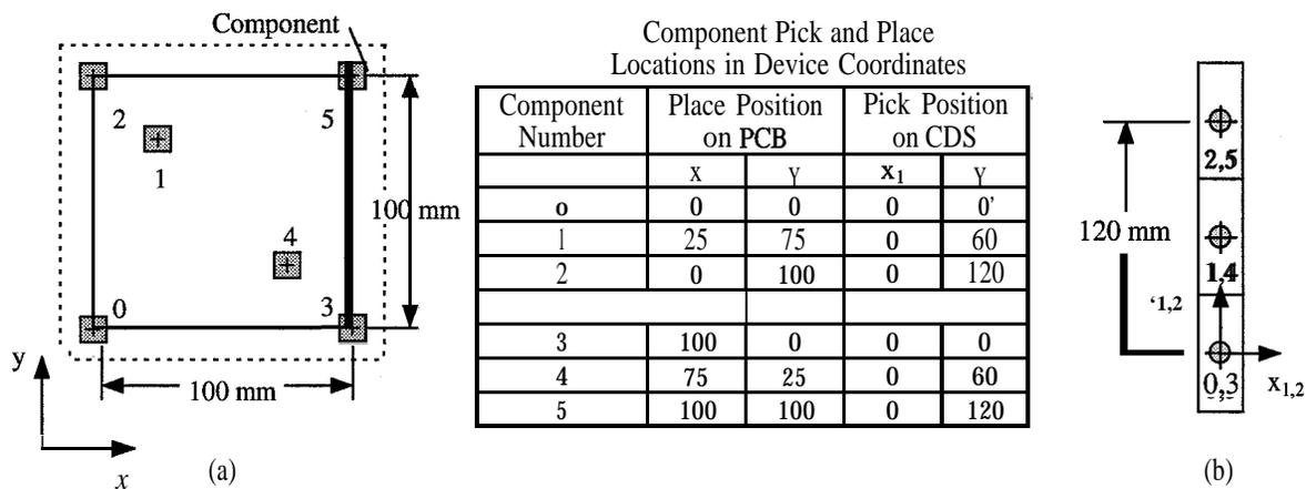
Figure 3: (a) The PCB with component positions. (b) One of the two identical CDSs.
