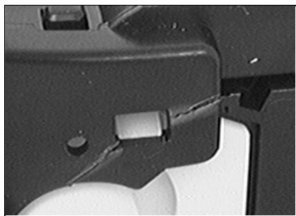
Figure 3. Cracked Slot in Toner-cartridge Housing.
