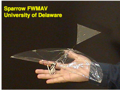
Figure 5: Sparrow Flapping Wing Micro Air Vehicle [21]
