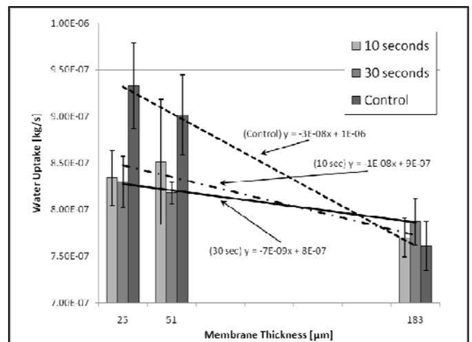
Figure 6. Water uptake for flow reversal (10 & 30 sec) and membrane thickness (Control – NR-211, NR-212, N-117).
