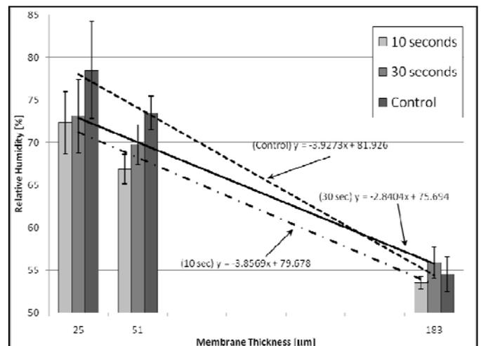
Figure 7. Outlet relative humidity for flow reversal (10 & 30 sec) and membrane thickness (Control – NR-211, NR-212, N-117).
