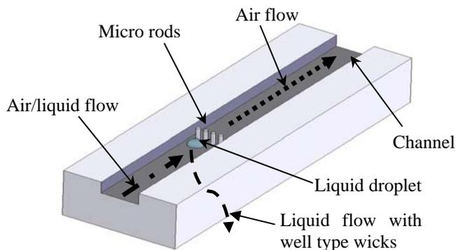
**Figure 13. Trapping liquid with hair-like features.**
