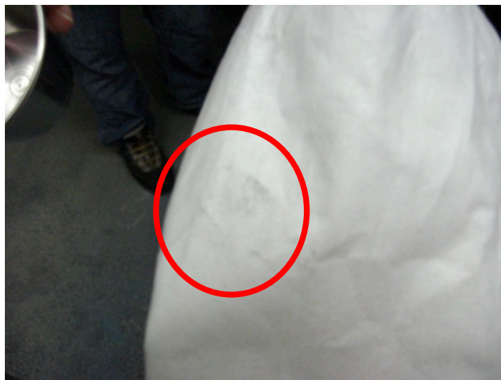
Fig 5 : Collected dust out of coil 7 on white rag
