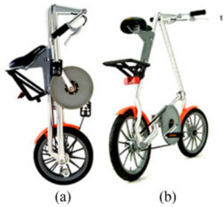
Fig. 5. (Color online) Strida folding bike. Images (of earlier model) used with permission ( http://www.strida.com ). (a) Folded state and (b) riding state.
