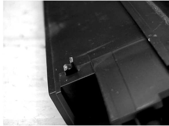
Fig. 6. Broken Protrusion: Male Snap-Fit Lock.
