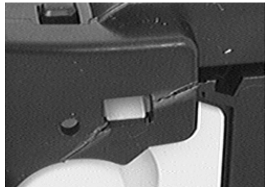
Figure 2. Extra hole in toner-cartridge housing.
