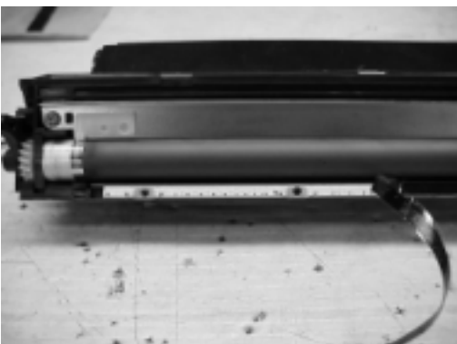
Figure 1. Unglued seal on toner cartridge.
